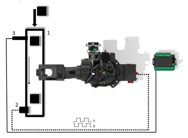
In the above application, the user gives the workpieces (cubes) at the beginning of the conveyor belt, when the sensor triggers, a point is saved, to which the robot then goes and picks the detail at the same time synchronizing with the conveyor belt. It then puts the items in a different location.
