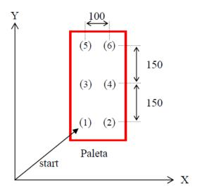
In the following example, items are palletized in order from (1) to (6). Enter the initial settings listed below. The palette is positioned parallel to the robot's global coordinate system.
