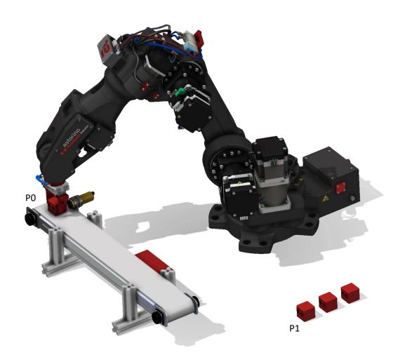
In order for the above application to work properly, the workpieces should be given in the same orientation and position on the conveyor belt (relative to the width), this can be done by designing appropriate bumpers that will automatically position the detail in the middle of the conveyor belt
