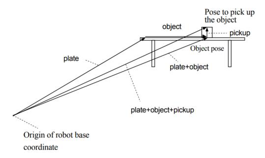
If you repeatedly use the value of a compound transformation, use the POINT command to reduce the time it takes to calculate the value of the compound transformation. For example, to approach the "pickup" position, and then to go to this position, you can type:
