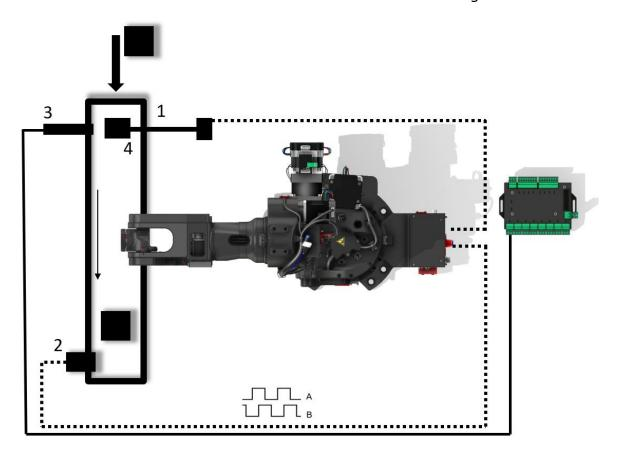
In the above application, the user puts workpieces (cubes) at the beginning of the conveyor belt, when the sensor triggers, the camera is activated, which detects the object on the conveyor belt and sends the coordinates to the robot. A saved point is used to determine the location of the workpiece. The robot then goes and picks up the cube while synchronizing with the conveyor belt. It then puts the picked up items in a different location.
