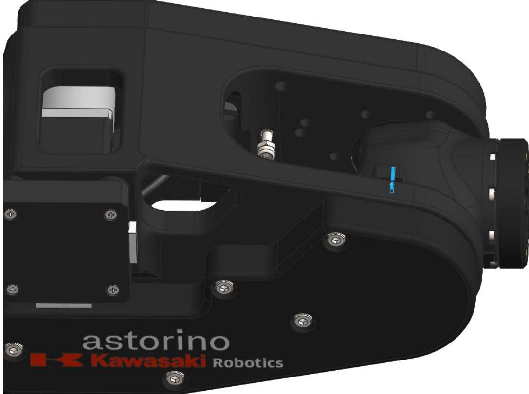
You can use 1 or 1.5mm drill or 1.5mm hex alan wrench to find zeroing position (not necessary) – remove the JT6 motor cover
