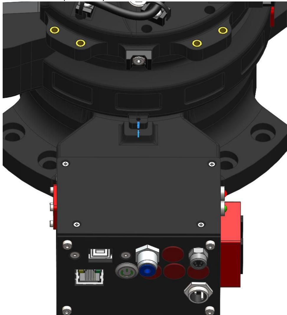
You can use 2.5mm drill or 2mm hex alan wrench to find zeroing position (increases the zeroing accuracy)
