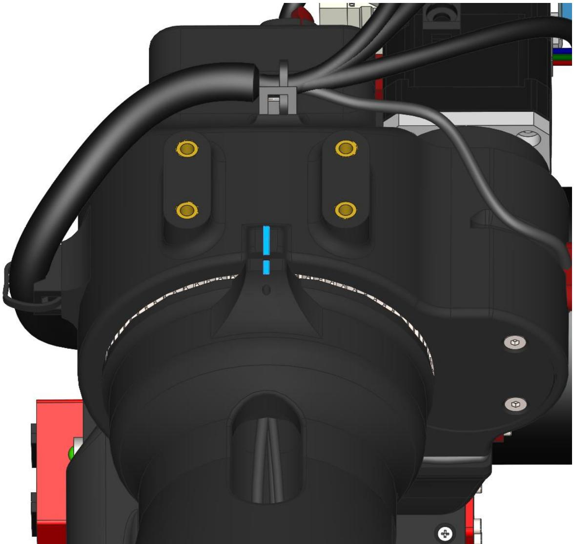
You can use 2 or 2.5mm drill or 2mm hex alan wrench to find zeroing position (not necessary)
