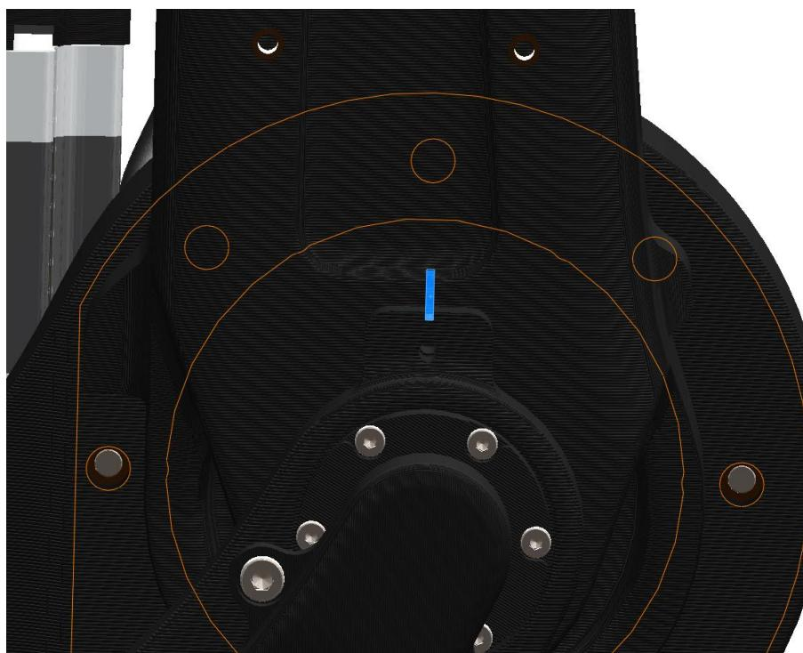
You can use 2 or 2.5mm drill or 2mm hex alan wrench to find zeroing position (not necessary)
