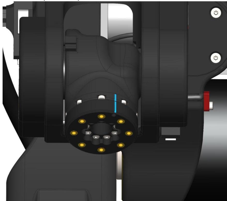
You can use 1 or 1.5mm drill or 1.5mm hex alan wrench to find zeroing position (not necessary)
