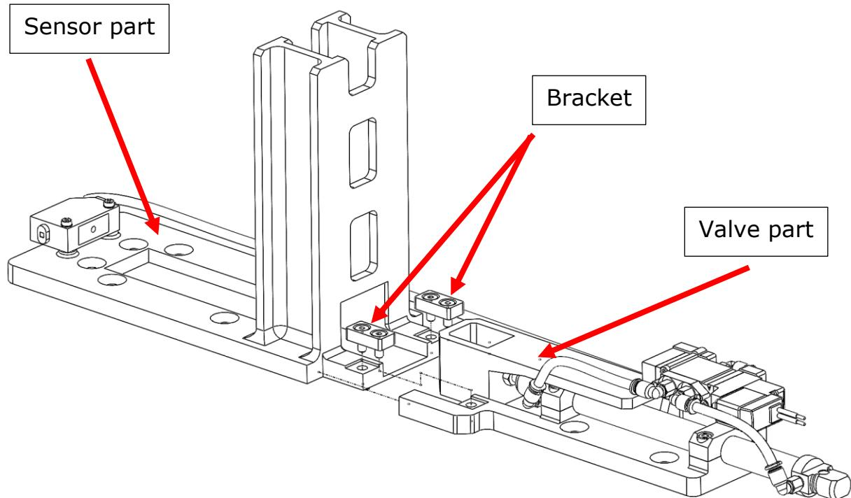
Connect two sides with a rectangular brackets and four DIN7991 M3 screws.
