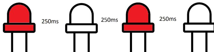
Turn off the robot and turn it on again. This is an error from the SD card inside robots base, CPU was not able to restart the card after firmware update. Resetting the power solves the problem.
