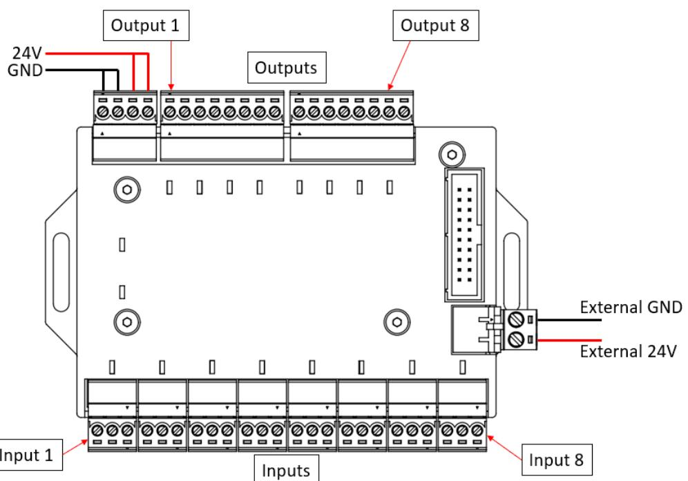
A total of 8 24V inputs and 8 24V outputs can be connected.
