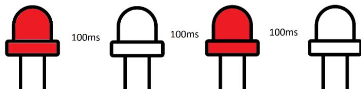
This means that the robot needs to update the data on the SD card. The procedure will perform automatically. When the procedure is complete, the red LED will turn off. And when connected to the computer, there will be a message that the SD card data repair/update procedure is complete
