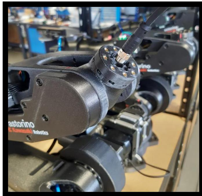
The cable from the gripper should be routed through the 6th axis and the 4th axis arm.
