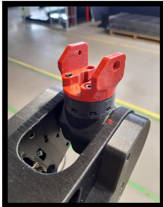
The fastener must be screwed to the robot flange using M3x8 cap screws.
