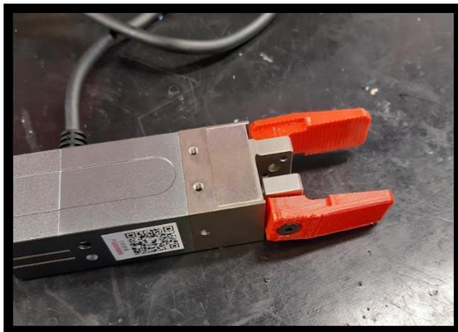
The jaws must be attached to the electric gripper using M4x12 taper screws.
