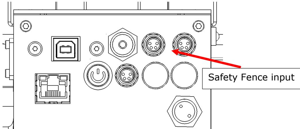
Emergency stop circuit is two channel, to connect external safety device follow listed below diagram.
