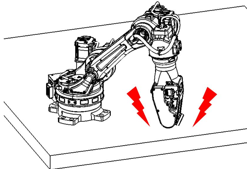
**During power loss when there is heavy gripper installed JT5 might make a sudden movement!**
