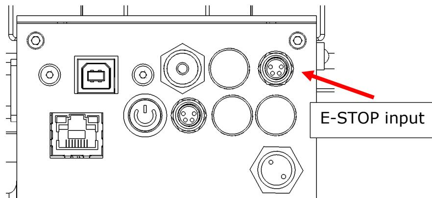
Emergency stop circuit is two channel, to connect external safety device follow listed below diagram.
