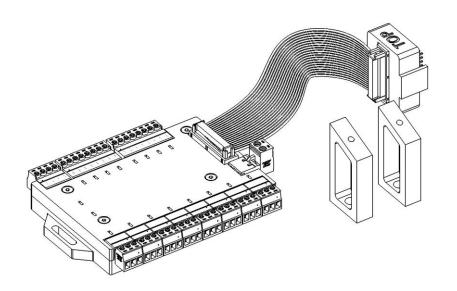
IO Module, ribbon cable, IO adapter, stand
