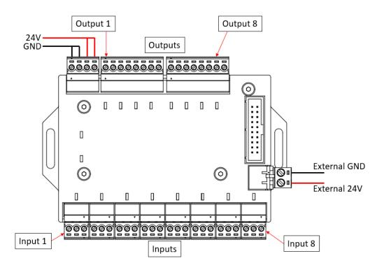
A total of 8 24V inputs and 8 24V outputs can be connected. Each output provides 300mA current (approx. 7.2W output power).
