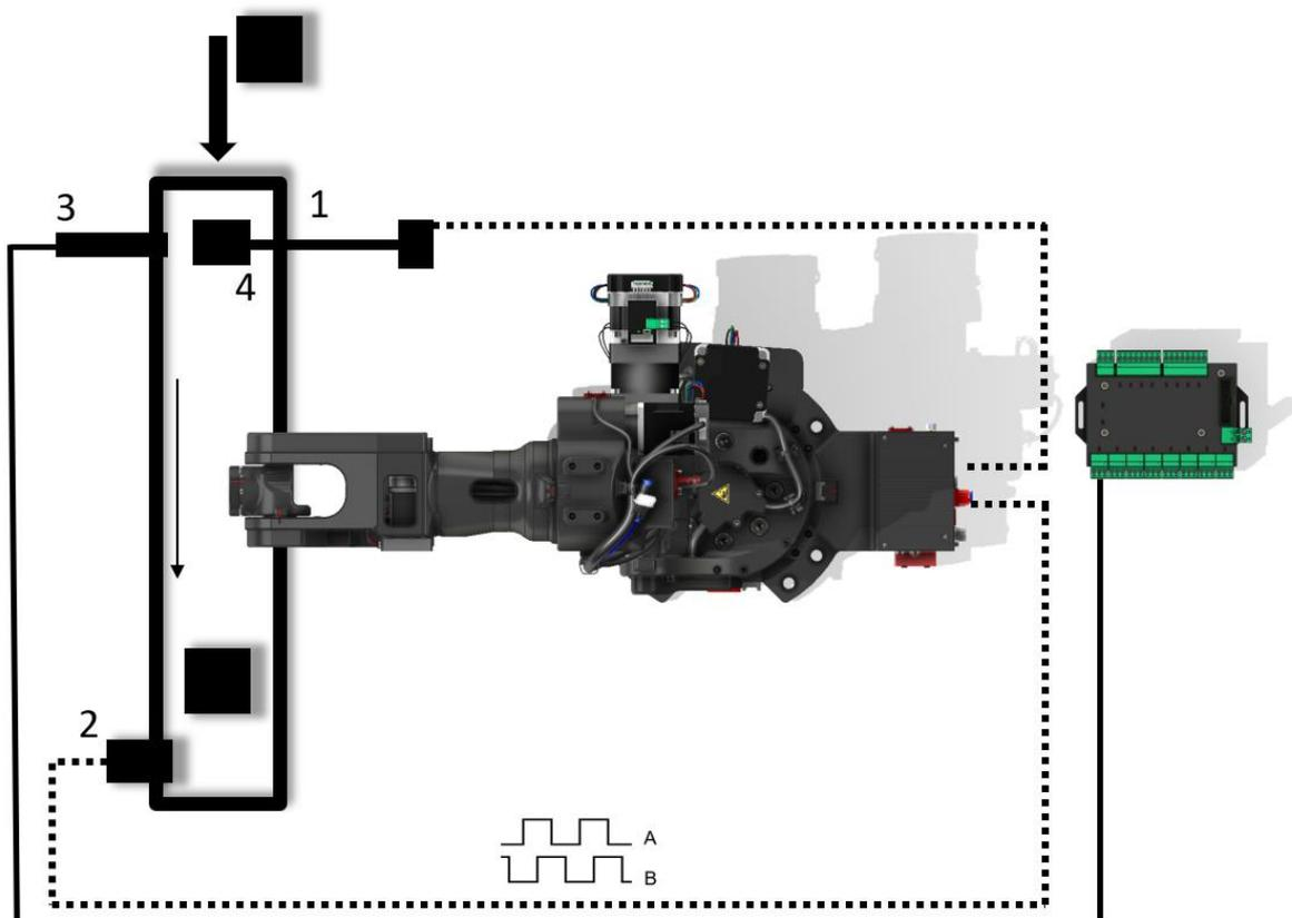
In the above application, the user puts workpieces (cubes) at the beginning of the conveyor belt, when the sensor triggers, the camera is activated, which detects the object on the conveyor belt and sends the coordinates to the robot. A saved point is used to determine the location of the workpiece. The robot then goes and picks up the cube while synchronizing with the conveyor belt. It then puts the picked up items in a different location.
