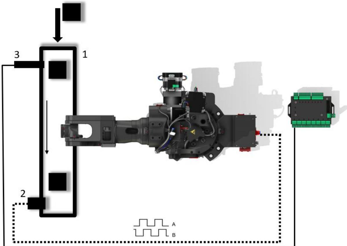
In the above application, the user gives the workpieces (cubes) at the beginning of the conveyor belt, when the sensor triggers, a point is saved, to which the robot then goes and picks the detail at the same time synchronizing with the conveyor belt. It then puts the items in a different location.
