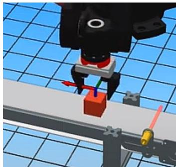
Then switch mode to CONV, turn on the conveyor so the belt is moving and press one of the JOG buttons. Robot should move in synchronization with the belt.
