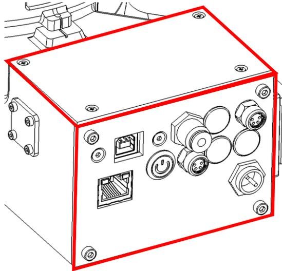
3. Insert the included M8 plug through the hole in the rear panel located next to SERIAL communication connector.
