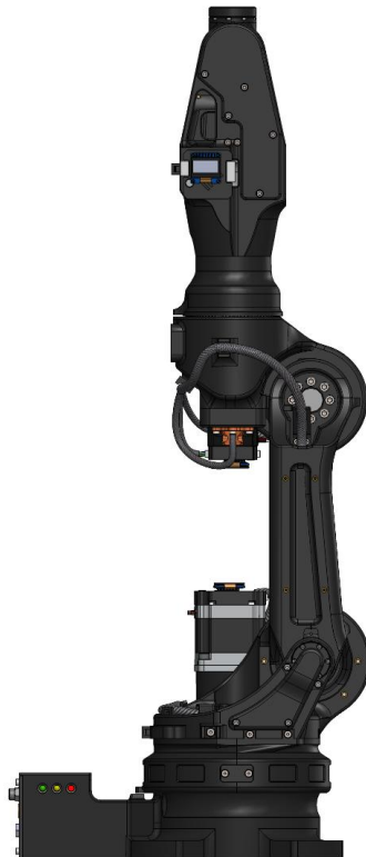
Zero position of the Astorino robot arm.
