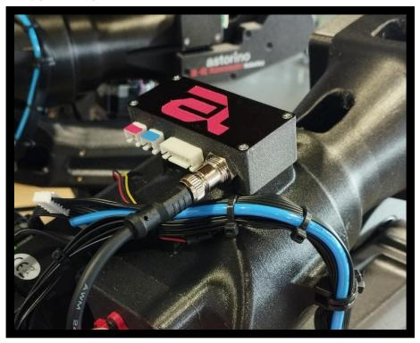
The gripper cable has to be plugged into the arm id.
