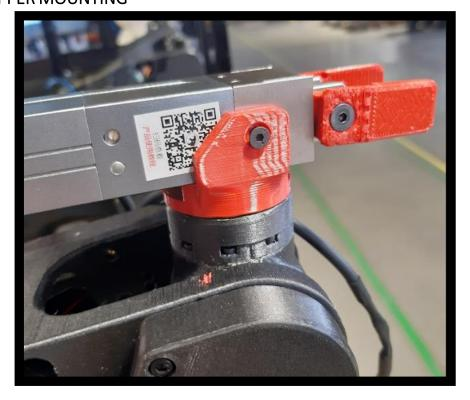
The electric gripper must be screwed to the flange-mounted component using M3x8 tapered screws.
