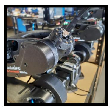
The cable from the gripper should be routed through the 6th axis and the 4th axis arm.
